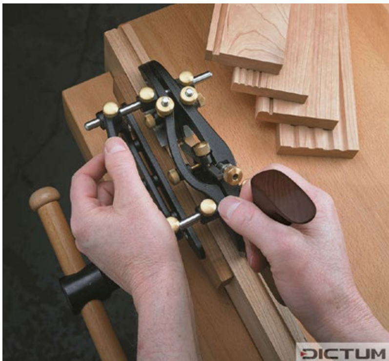
Veritas Router Plane, high-carbon steel Blade
