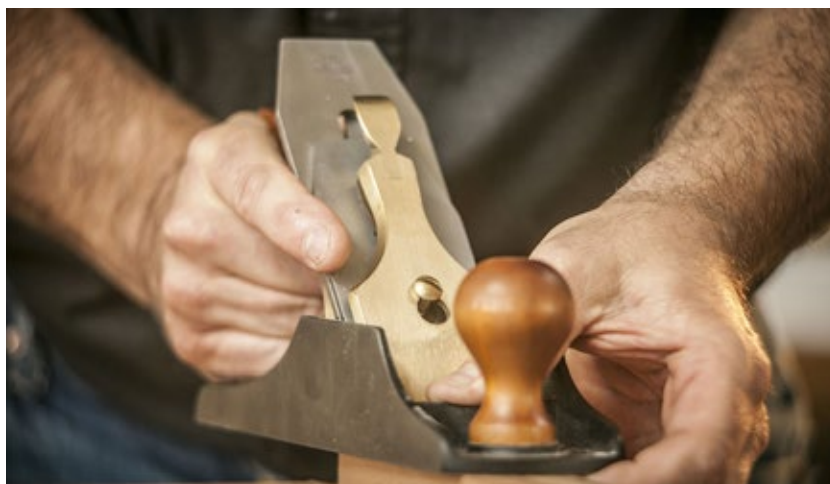
Lie-Nielsen Smoothing Plane No. 4, Spheroidal Cast Iron
